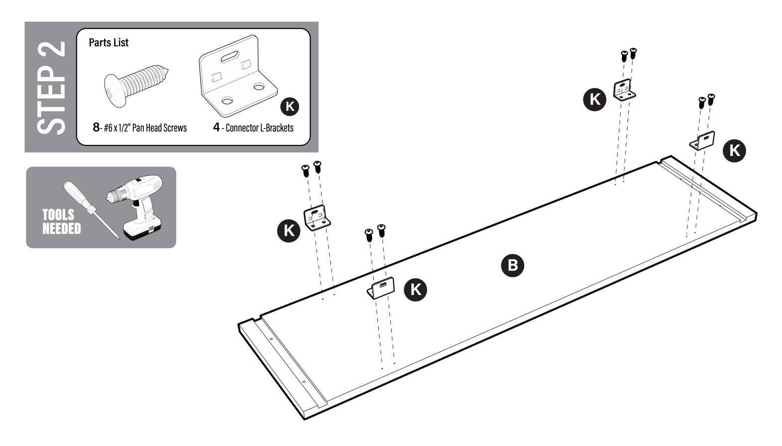
Place Back Panel (B) on a flat smooth surface and install (4) tan RTA L-Brackets (K), as shown, using (8) #6 x 1/2" Pan Head screws.
