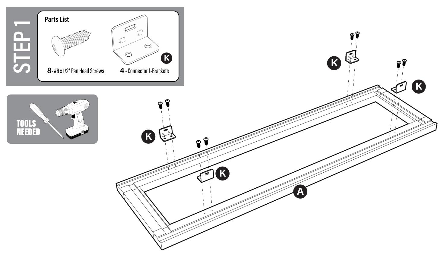
Lay Frame (A) face down on a smooth flat surface, install (4) tan RTA L-Brackets (K), as shown, using (8) #6 x 1/2" Pan Head screws.
