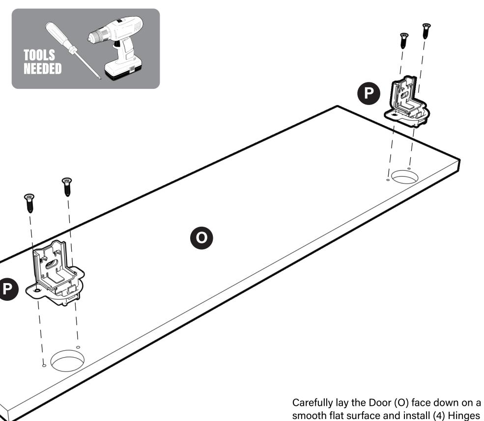
Carefully lay the Door (O) face down on a smooth flat surface and install (4) Hinges (P) using (8) #6 x 5/8" Countersunk Flat Head screws.
